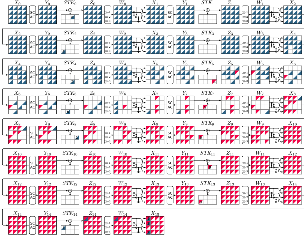
Figure 5: 15-Round boomerang distinguisher for SKINNY-64-192 from the tool in [HBS21].
